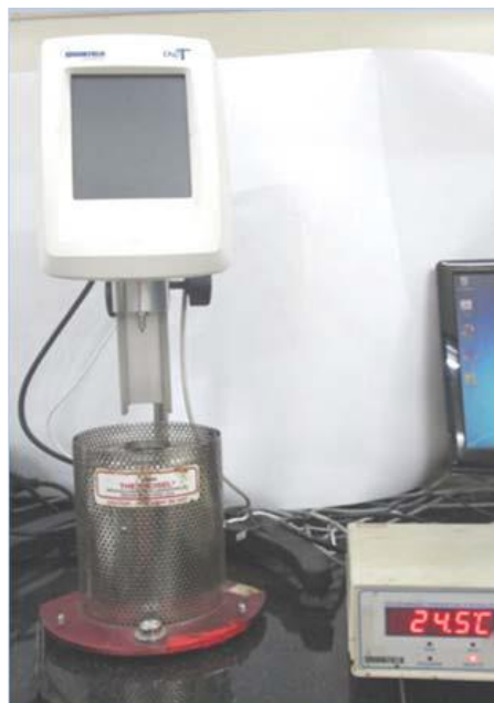
Figure 5.3 Brookfield HA DV II + Pro viscometer (Asphalt Laboratory, IITM)
